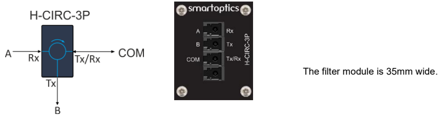
Figure 52: 3-port circulator icon and front plate
