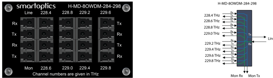
Figure 58: H-MD-8OWDM-284-298 icon and front plate
