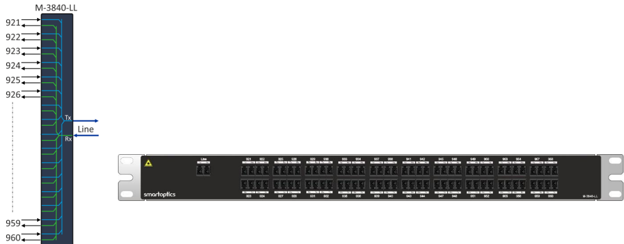
Figure 36: M-3840-LL icon and front plate
