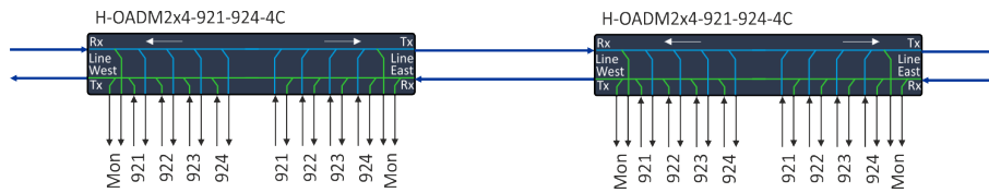
Figure 44: Two H-OADM2x4-921-924-4C filters connected in a bus configuration.
