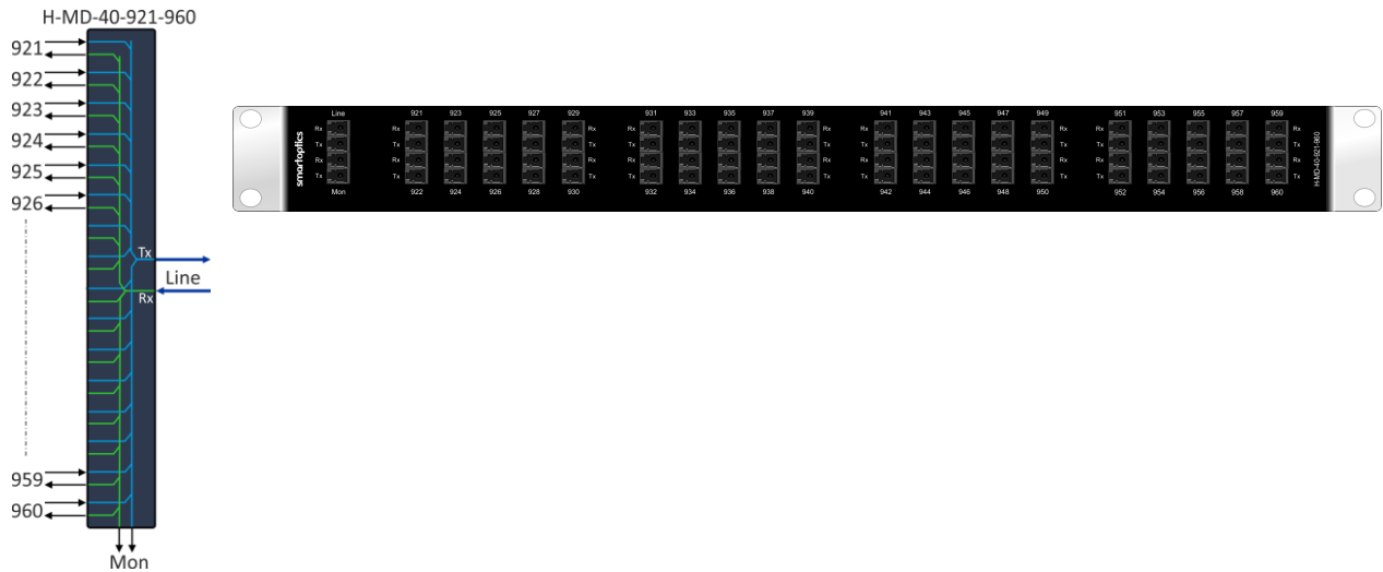
Figure 35: H-MD-40-921-960 icon and front plate
