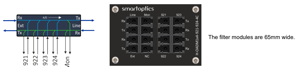
Figure 41: H-OADM1x4-921-924-4C icon and front plate
