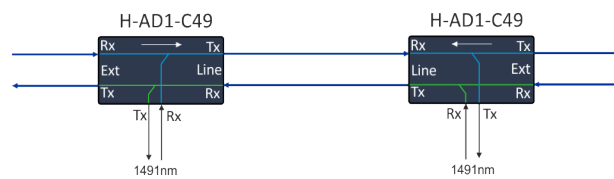
Figure 22: H-AD1-C49 connection example
