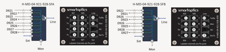
Note row dependent location of Tx and Rx ports. This is due to the usage of duplex LC connectors.
