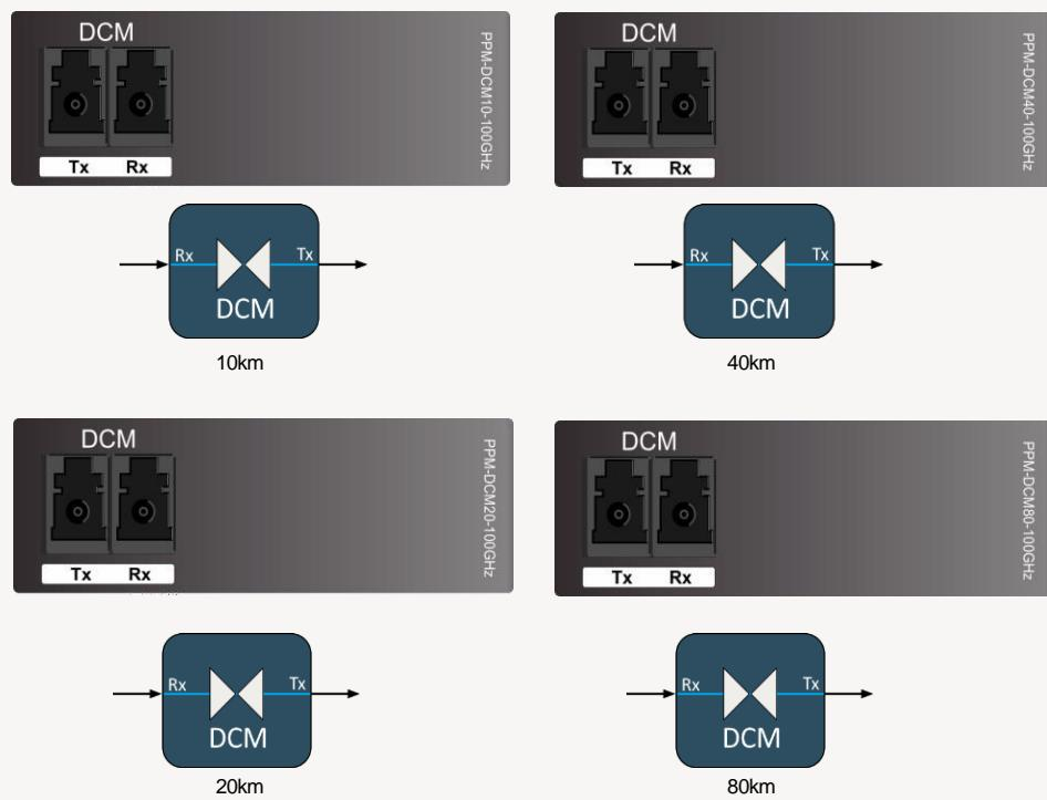
The DCM modules contain a channelized Fiber Bragg Grating (FBG) dispersion compensating component that provides the opposite dispersion of a 10km, 20km, 40km and 80km SM-fiber length, respectively.
