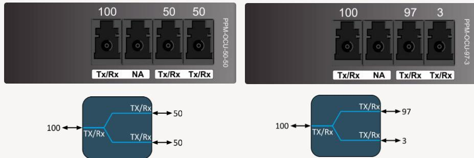
The OCU modules are C-band optical couplers where the signal is split or combined with the ratio 50% - 50% and 97% - 3%, respectively. The 97/3-coupler is intended for cases where a smaller portion of the optical signal is to be connected to e.g. an Optical Channel Monitoring (OCM) function.
