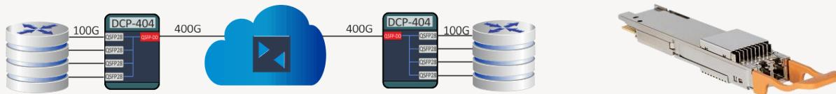
OpenZR+ is currently only defined for amplified line systems. OIF 400ZR is defined for both amplified as well as un-amplified configurations. The Application Mode 2 (OIF app code 0x02) corresponds to the un-amplified OIF 400ZR configuration.
