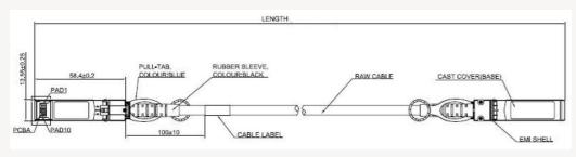
Minimum bend radius AWG30: 23mm
